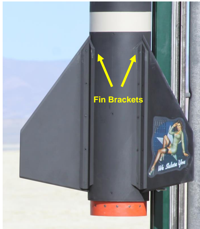
Figure 31 – Example Inclined Flat Plate Protuberances, fin brackets.
