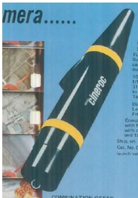
Figure 30 – Cineroc camera shroud, modeled as a Streamlined – With Base Drag Protuberance.
