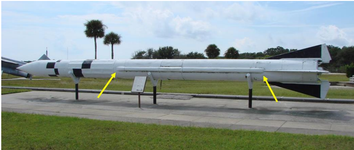
Figure 28 – Example Streamlined – No Base Drag Protuberance, a missile raceway.
